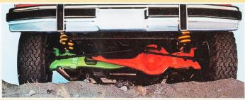
Tough new Twin-Traction Beam independent front suspension eases wheels over bumps separately to cushion the vehicle, smooth the going, and improve off-road control. It's smooth on the road—tough off the road.
