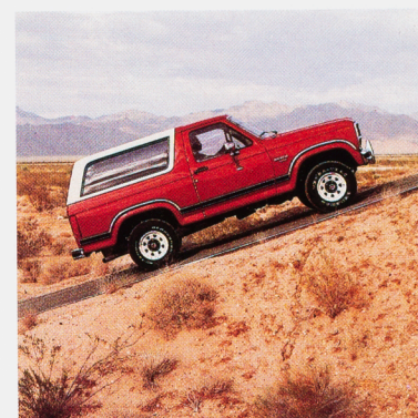
A 30% grade is used to test Bronco's parking brake hold under a full load.
